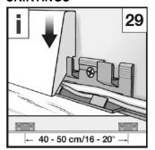
For the perfect finish, fasten the skirting boards at a distance of 40 - 50 cm to the wall and put on the matching skirting boards.
