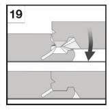
Insert a second panel lengthwise into the groove profiling of the preceding panel areas and slide it to the left at an angle of 20 ° to the already laid panel. Then
