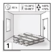
Store the planks in the unopened packaging at room temperature horizontally in the room for at least 48 hours before installation. Before, during and at least three days after installation, the following room climate conditions must be ensured:room climate:
