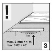
The substrate for laying the designfloor must be such that the floor can be laid according to the instructions. As underground are u.a. mineral substrates (such as screed, concrete, asphalt), which must be absolutely level, dry, clean and stable.
