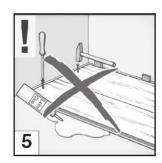
The flooring is laid floating and must not be glued, screwed, nailed or otherwise fixed to the subfloor.
