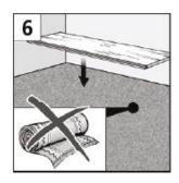
Carpets must always be removed. The carpet underneath the flooring causes a resilient movement and too much when walking on the surface. The pressure in the edge area destroys the tongue and groove connection and leads to a joint formation.
