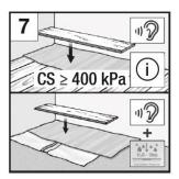
For wooden substrates no PE foil may be laid. Before laying on mineral subfloors (concrete, screed, etc.), a suitable vapor barrier film must be installed to protect against moisture. On all substrates, a suitable underlayment is necessary. (pressure stress min. 400 KpA, e.g.1016 Soft Sound, 1009 V-Sound or 1020 V-Premium Sound). The insulation underlay is laid on "impact" and fixed with Alu Tape, i.e. not overlapping. It must be ensured that the joints of the insulation underlay are not
