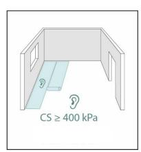
The use of a suitable impact sound insulation for vinyl floors is necessary. Please use an impact sound insulation with a pressure load of min. 400 kPa.
