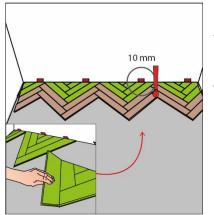
Put the adjusted rows (in the picture green marked) into place. If you use version 1, connect the cut starting panels to form triangular shapes. Start installing the triangles from the left corner. It is recommended to use glue to fix the smallest parts (click-connections) of the triangles. Make sure that you leave a gap of 10 mm to the wall.
