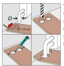
Where, for example, heating pipes protrude from the floor, please first cut the panel to the correct length, then place the panel piece next to the actual slot and measure and mark the cut-outs with a tape measure. Please always keep in mind the minimum distance of 10 mm for the expansion joint. Now you can drill out the marked areas and saw the panel to size. Then place it behind the heating pipe and join it tightly with the panel.
