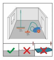
The substrate must be crack-free, clean, tension/compression resistant and completely dry (VOB, Part C, DIN 18365). Before laying, remove all old floor coverings from the subfloor as far as they may affect the evenness of the subfloor. The evenness of the substrate should not deviate by more than +/- 3mm on 1m (DIN 18202).
