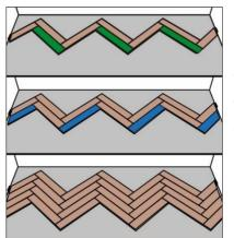
Continue from the left to the right and install all the A-panels in the second row. Now work in the opposite direction, from the right to the left and install all the B-panels in the second row. To do this, press down on the short side of the plank until it engages completely. Finish with a piece of panel cut to size. Install additional rows to complete four full rows.
