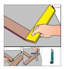
Measure and cut the end panels to size using a fine-toothed saw. Finish the first row with the cut end panels. Make sure that you leave a gap of 10 mm to each wall.
