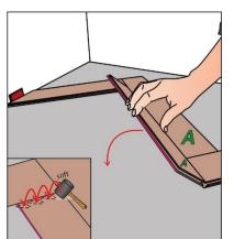
Start the next row with an A-panel. Place the new panel against the previous row and fold down. To do this, press down on the short side of the plank so that the click connection engages completely. If necessary, tap lightly with a rubber hammer.
