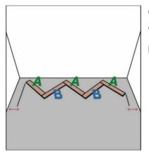
Check the first row of panels is centered along the starting wall. Make sure that the distance to the walls on both sides are less than the length of one panel. If not, add a panel at the right side.
