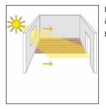
Lay the boards lengthwise to the main light source and thus towards the incoming light. The boards should be installed/laid from left to right. The boards must be floating.
