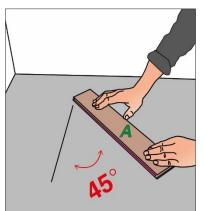
Choose a wall to start at and begin installing at the left corner. Start with an A-panel and place it with its long side marking facing the left wall at an angle of 45 degrees. Make sure that the distance between the left wall and the panel ist less than the length of the panel.
