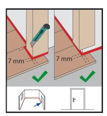
Wooden door frames can be shortened. Place a panel with the decor side down against the frame. Now shorten the door frame with a suitable saw along the panel. Then simply slide the panels under the door frame with the decor side up. In the case of door frames that cannot be shortened, cut the panel to size accordingly and observe the minimum 7mm circumferential distance for the expansion joints.
