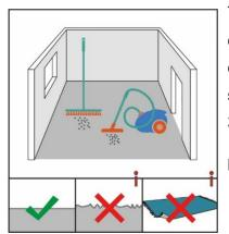
The substrate must be crack-free, clean, tension/compression resistant and completely dry (VOB, Part C, DIN 18365). Before laying, remove all old floor coverings from the subfloor as far as they may affect the evenness of the subfloor. The evenness of the substrate should not deviate by more than +/-3mm on 1m (DIN 18202).
