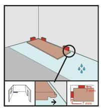
**NOTE FOR CHECK COMFORT:** If you install CHECK comfort with integrated cork underlay on a screed floor, please remember the vapor barrier. Please fix the vapor barrier in advance with an AluTape.
