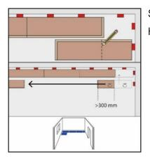
Start the next row with the remaining piece of flooring from the previous row. However, remnants should be at least 30cm long to ensure optimum stability.
