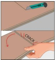
The custom-made panels are easily shortened with an angle and a carpet knife. The panel is then "broken over the edge".
