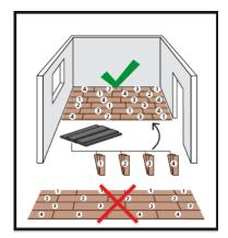
Before laying, check each individual board for colour and structure. It is advisable to mix several packages in order to obtain a uniform laying / sorting pattern. Note: Only use material from the same batch in a room.
