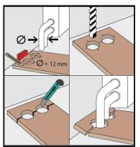
Where, for example, heating pipes protrude from the floor, please first cut the panel to the correct length, then place the panel piece next to the actual slot and measure and mark the cut-outs with a tape measure. Please always keep in mind the minimum distance of 7 mm for the expansion joint. Now you can drill out the marked areas and saw the panel to size. Then place it behind the heating pipe and join it tightly with the panel.
