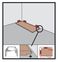
The first row is laid so that the spring of the head and long side faces the wall. Fix the first row with spacers (min. 7 mm) to the wall.
