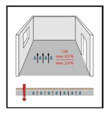
Check the humidity of the subfloor. The maximum permissible humidity for cement screed is 2.0%, for underfloor heating 1.8%. For anhydrite (calcium sulphate) screeds the maximum residual moisture is 0.5%, for underfloor heating max. 0.3%.
