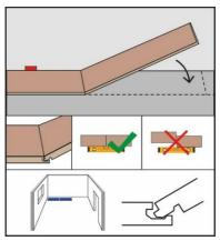
Click the front side of the panels into the previous panel at a slight angle.
